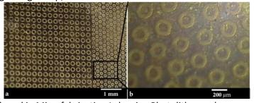
Micro patterns developed in Microfabrication Lab using Photolithography.
